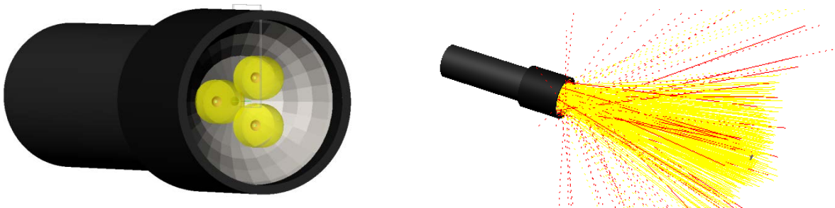
Figure 1. Left: Flashlight model in FRED. This model consists of the body, faceted reflector, and arrangement of three white-light LEDs. Right: Schematic ray trace of the flashlight. Rays reflected by the faceted reflector are shown in red.
